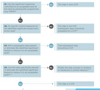
Figure 1 Example of a CCP decision tree - apply to each step where a specified significant hazard is identified
